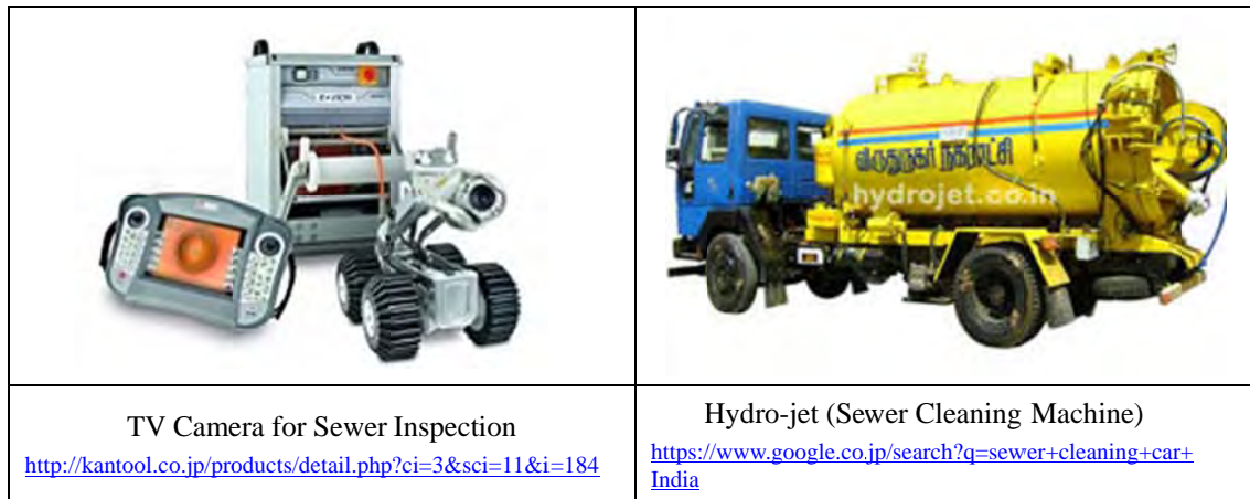
Figure 13.3.1 Images of TV Camera Investigation Car and Sewer Cleaning Car
