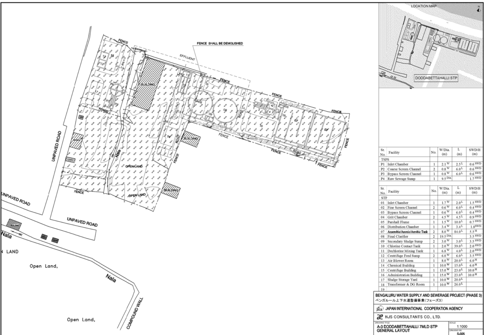
Figure 12.2.27 Layout Plan of Doddabettahalli STP
