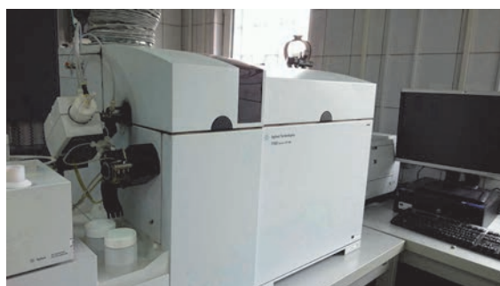
写真7-2-9 ICP-MS, Agilent Technologies 7700 Series
