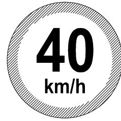
TS-3 SPEED LIMIT 40 KM/H SIZE: 600 MM DIAMETER
