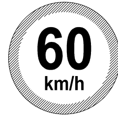
TS-2 SPEED LIMIT 60 KM/H SIZE: 600 MM DIAMETER
