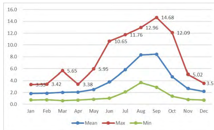
Figure 1-6: Mean, maximum and minimum water levels by month (1994 – 2015)
