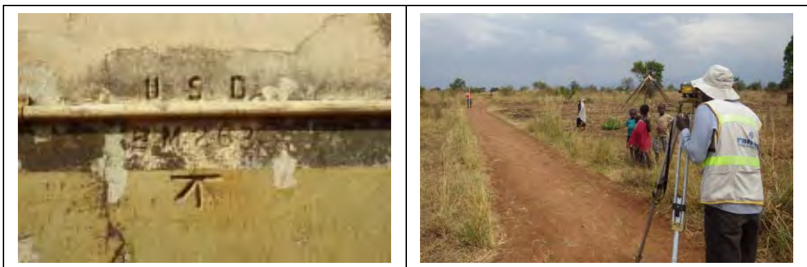
Figure 1.7 Left: BM263, Right: Leveling work
