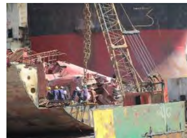
Lifting large blocks by crane (NK certified yard)
