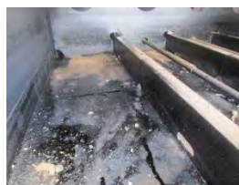
Oil still remaining inside fuel tank after
