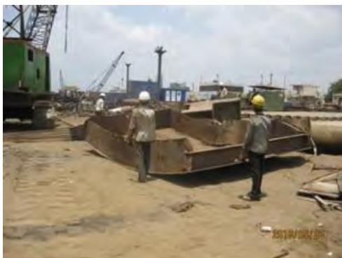
P.V-7 barge with sled shape
