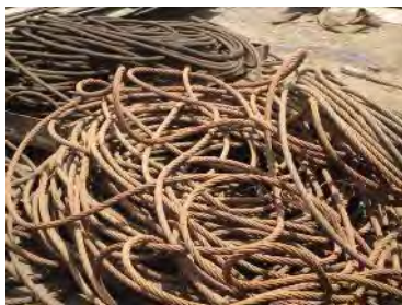
Lack of routine check of fixtures including winch line (Normal yards)
