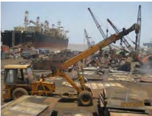
P.68 wheel crane distributing plates
