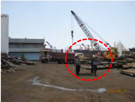
P.V-5 loading plates on truck, and carrying a plate on worker's shoulder
