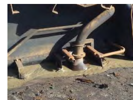
Water coming inside the fuel tank while the ship is waiting in inter-
