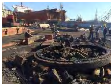
Oily parts and steel plates are stacked together (Normal yards)
