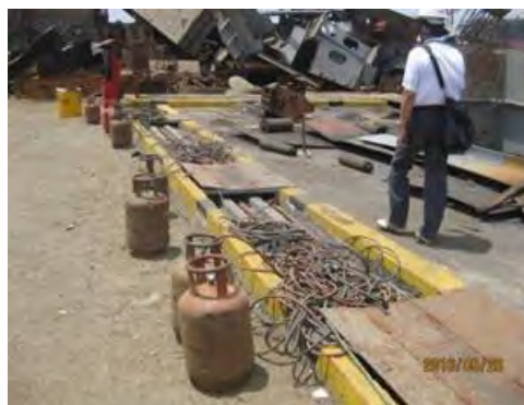
P.5 fixed supply pipe of oxygen gas and LPG gas bottles
