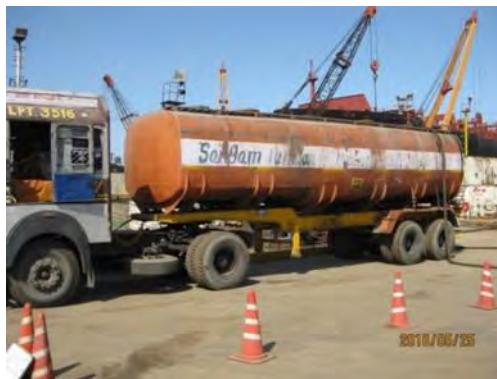
P.19 Tank truck for Oily Bilge
