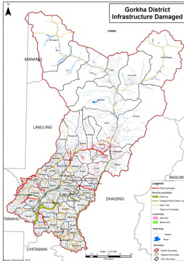
Figure. 3.17 Damaged Road from the Earthquake Source: Gorkha DDC 2015, prepared by JICA Project Team
