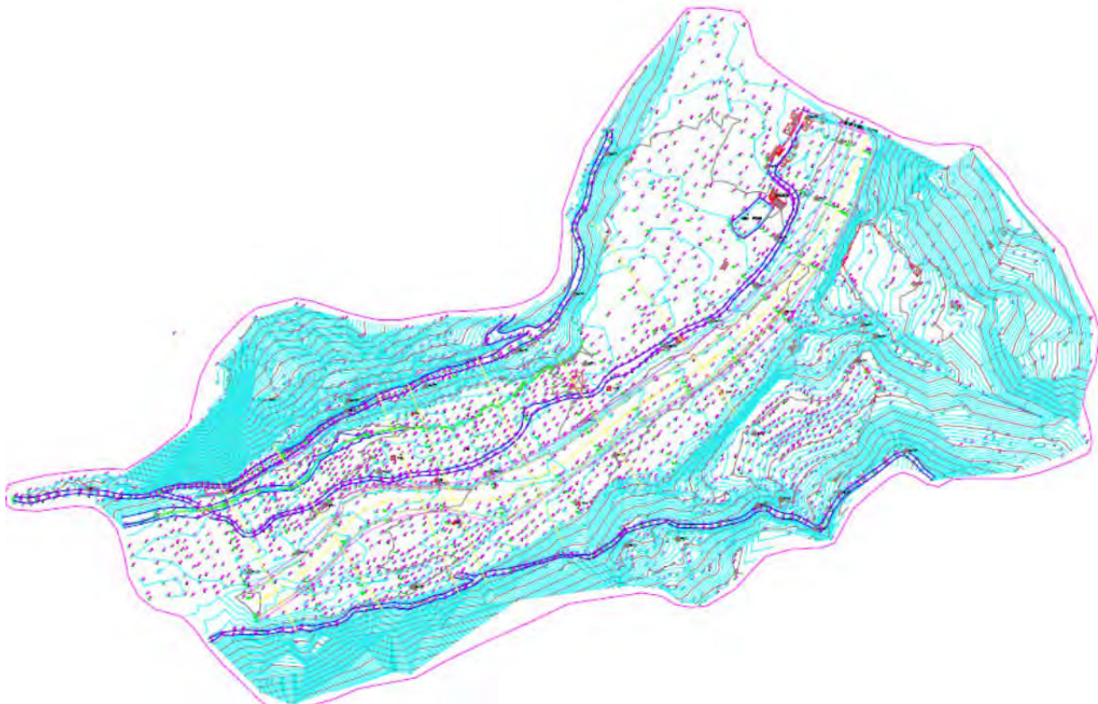
Figure 9.4.16 Topographic Map for Daraudi Khola Bridge Site
