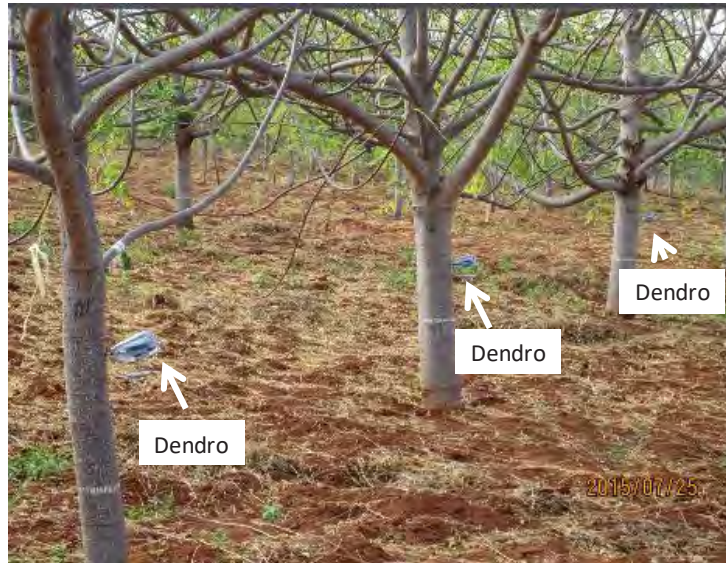
Photo2 Manual type of dendrometer installed to Melia clones at Tiva seed orchard.
