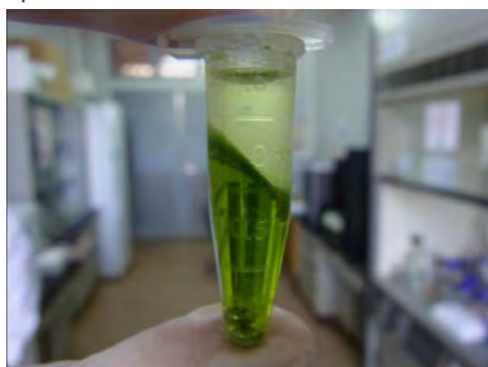
High purity DNA extraction by CTAB method
