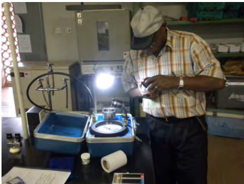
Photo 5 Measurement of xylem water potential using the newly introduced pressure chamber.
