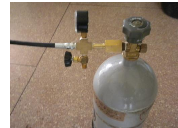
Photo 4. Air bomb and pressure chamber connection
