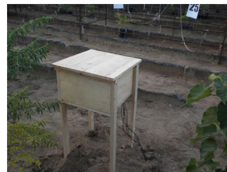
Photo 2. A box made of wood to store the water content meter and thermometer.
