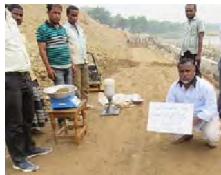
Ph20 & 21. Laying by Bulldozer & Field Density test by sand replacement method
