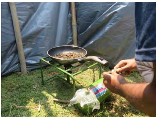
Photo 3.4.6 Measuring field water content (Frying Pan-Method)
