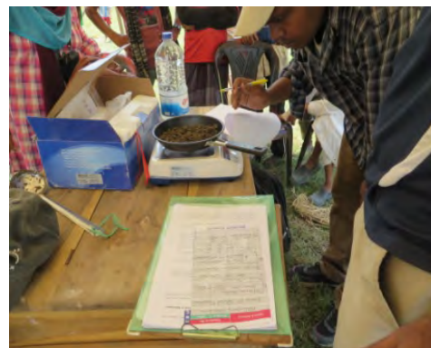
Photo 3.4.6 Measuring field water content (Frying Pan-Method)
