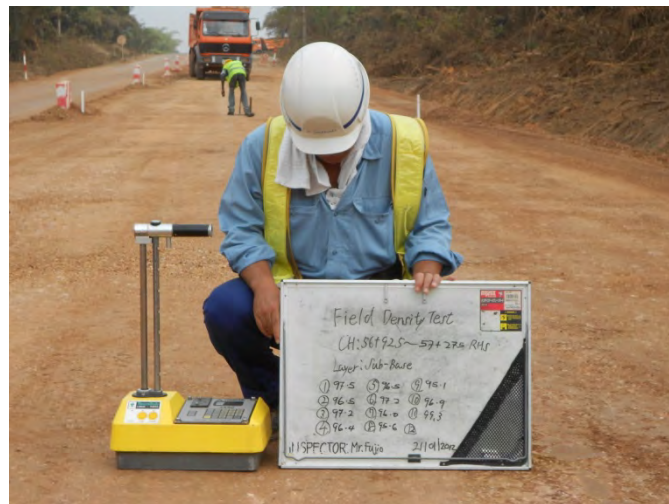
Photo 3.4.5 Field density test using an RI gauge
