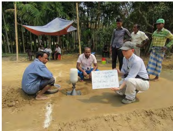
PhE. FD test of no.2 hole for 6 passes but from 5cm below the compacted surface.
