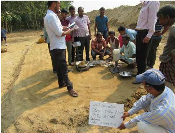
PhC. Field Density (FD) Test by sand-replacement method for 2 passes compaction
