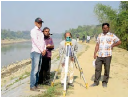
Photo 3.4. Cross Section Survey by TSS (JV) carried out at field on 13 & 14 December 2016.
