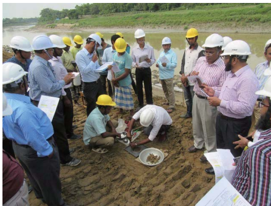
Photograph-5: Field Density Test (as of 02/Apr/2016)
