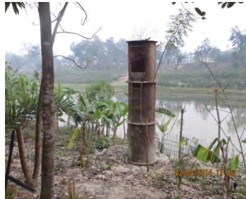
d. water-level gauge
