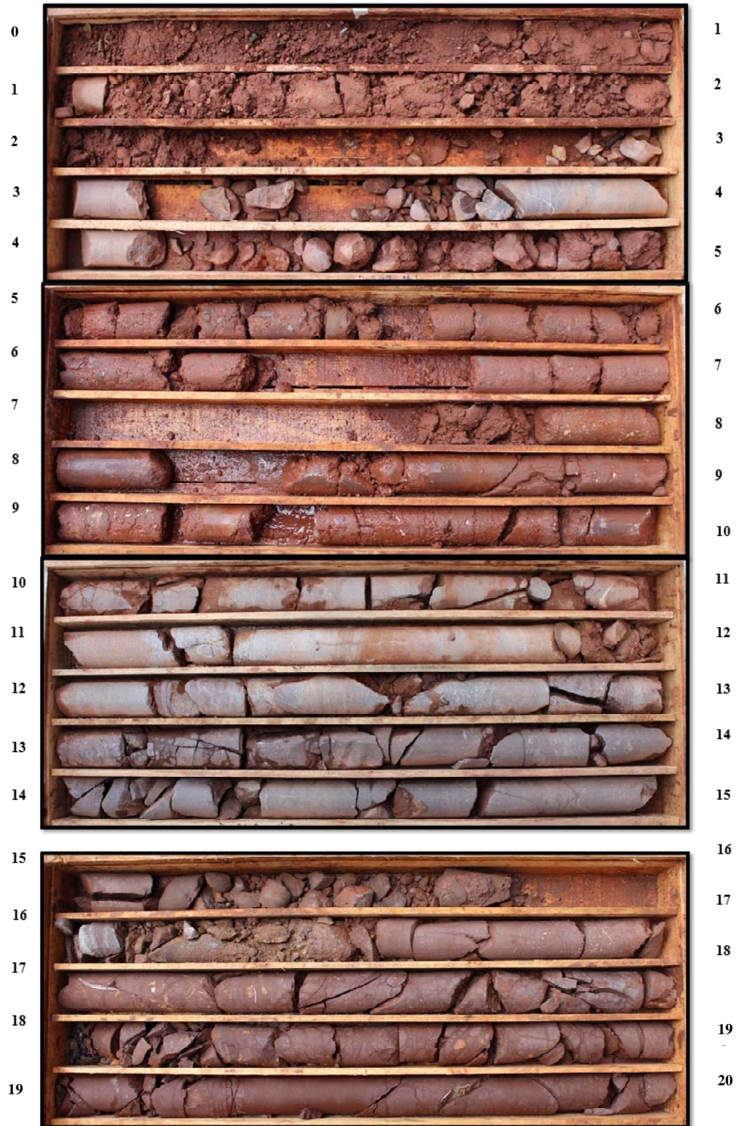
Figure 10. Complete core box D – Br3 borehole
