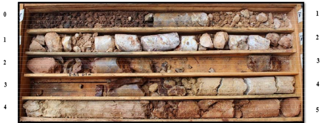
Figure 14. Complete core box E – Br3 borehole
