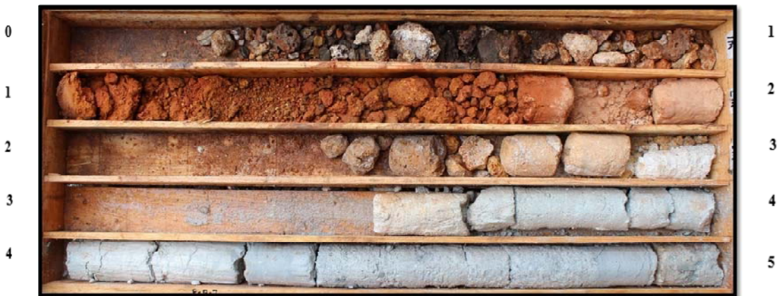
Figure 13. Complete core box E – Br2 borehole
