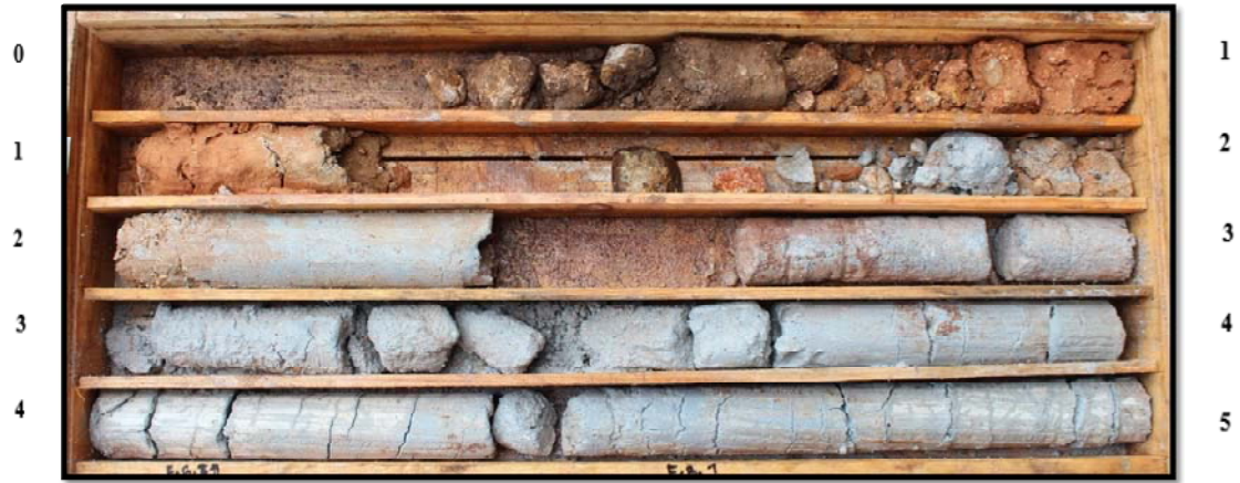
Figure 12. Complete core box E – Br1 borehole
