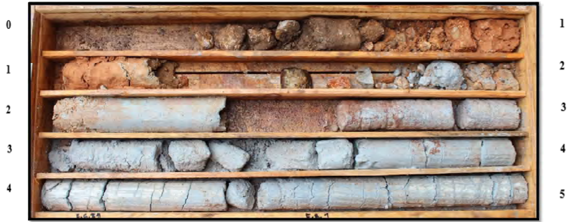
Figure 12. Complete core box E – Br1 borehole
