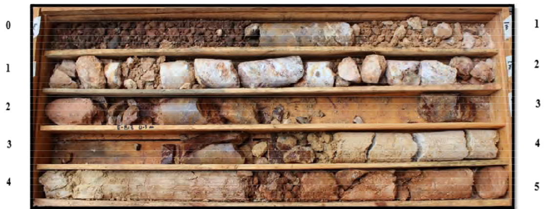
Figure 14. Complete core box E – Br3 borehole
