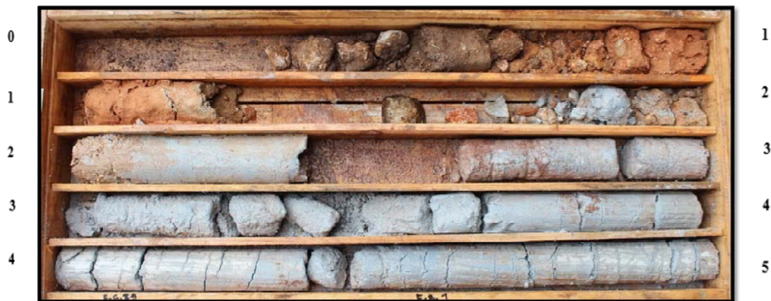
Figure 12. Complete core box E – Br1 borehole
