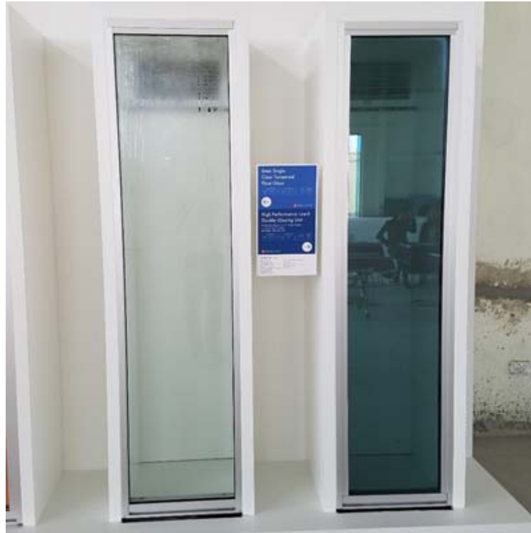
Figure 6-9 Energy saving glass demonstration equipment ((1) ref. (one sheet glass), (2) Low-E double glazing glass)
