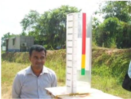
Simple Rain Gauge installed at Southern Highway
