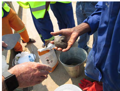
Checking the consistency of polymer cement mortar with bare hands; only in on-site OJT
