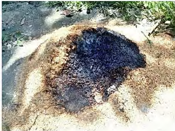
After some hours (2-4 hours), you will see black husks (pyrolyzed one) on the surface. Then, put the fresh ones from the bottom of the heap on to the top (gently mix).
