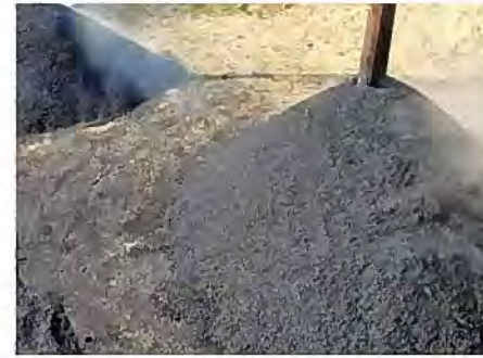
All the husks became black (pyrolyzed); then pour water to extinguish fire.
