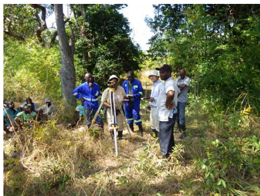
Practice on surveying with auto-level
