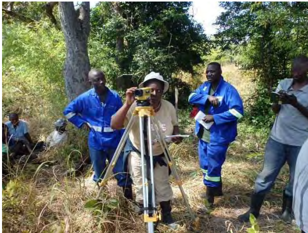
Field Practice: The TSBs actually starts surveying the topographic condition in the sample site to know the site is suitable to construct the permanent weir.
