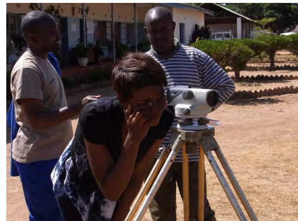
Practice on Dumpy Level: As a refreshment of what they might have learned in the college, TSB officers practice how to use dumpy level.
