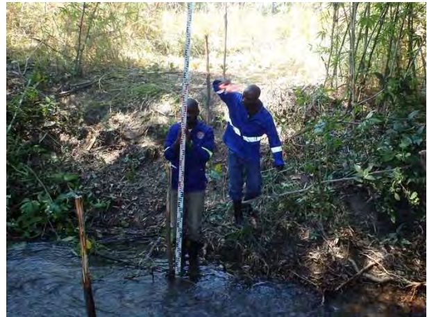
Field Practice: The amount of river flow is simultaneously measured to know it the amount of water is enough for irrigated agriculture planned.
