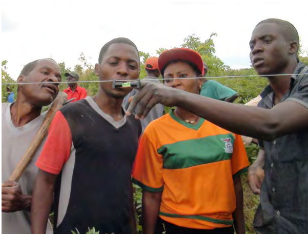
Field Practice on Canal Alignment: Looking at the spirit-line level, the direction of canal alignment is adjusted. "Pole-holder" needs to move according to the direction of the "level reader".
