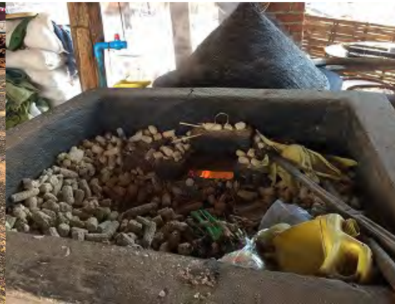
Photo II -28 Drying heater for sunflower seeds (Corncobs are used to compensate for the lack of firewood.)
