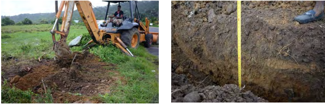
Figure 1-20 Photos of test pit survey at Cul-De-Sac bridge
