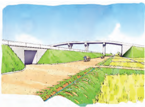
Under-Pass Culvert, Over-Pass Bridge and Frontage Road along Embankment Section
