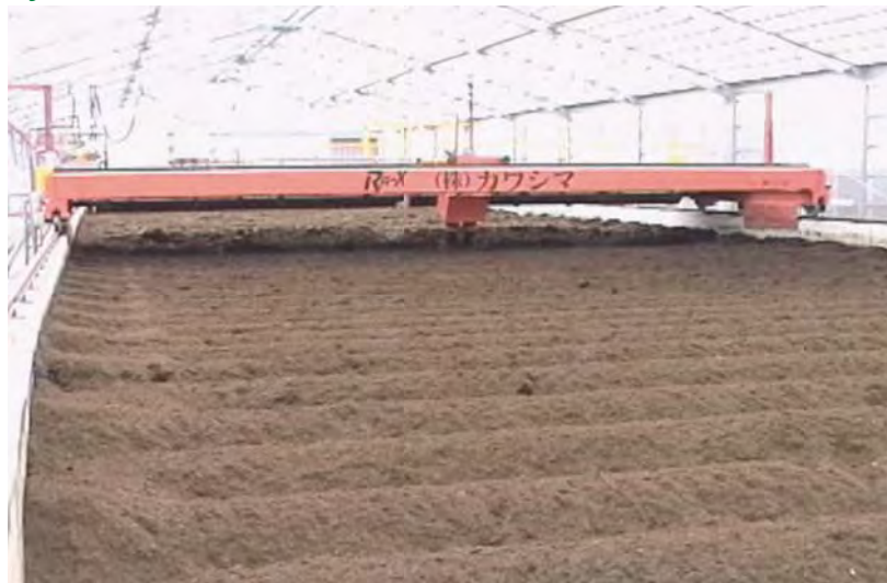
Simultaneous Treatment of Solids and Sewage by RA-X
