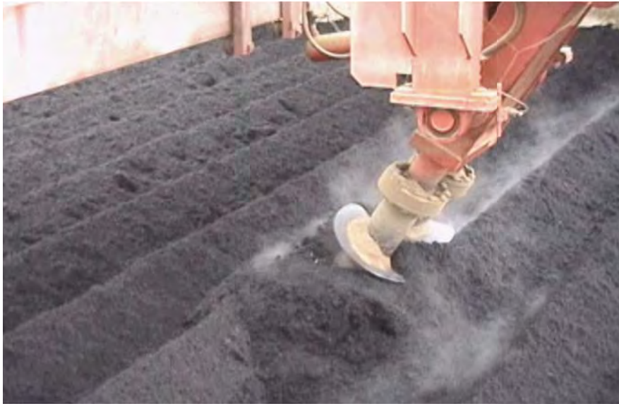
Screw type automatic stirring system “RA-X”
