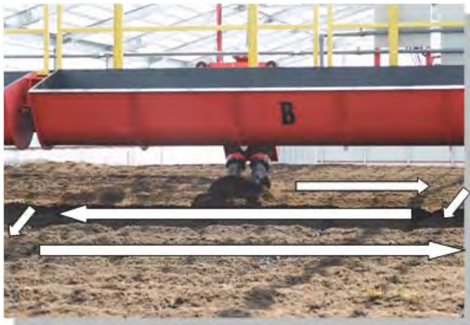
“RA-X” Automatic Stirring System, Showing Appearance of Stirring Shift Movement along Crank Path
