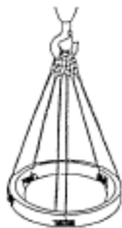
Six-rope, single-turn slinging
