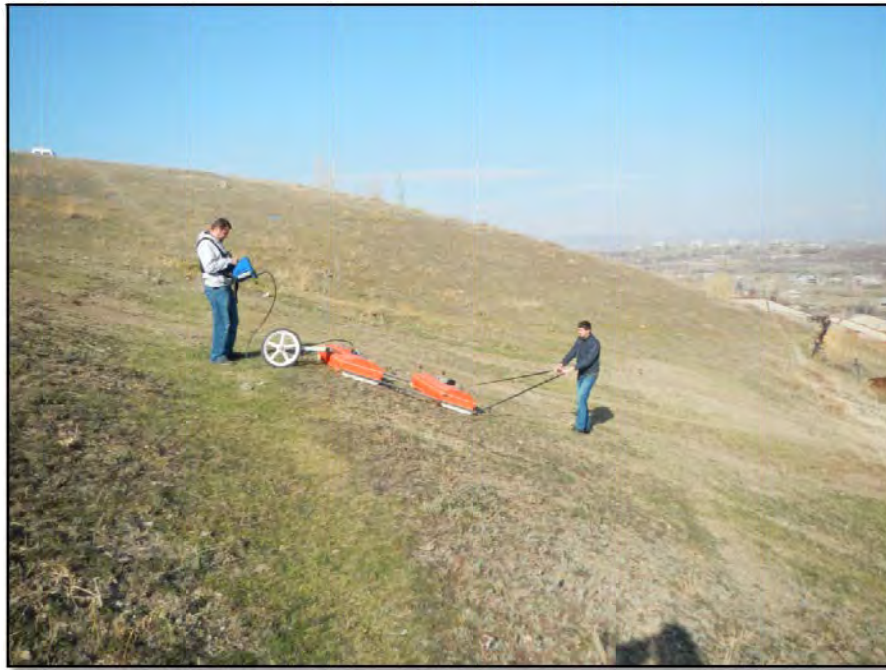
Figure 2.1: The recording device of the SIR-3000 geo-radar system and the process of field measurements
