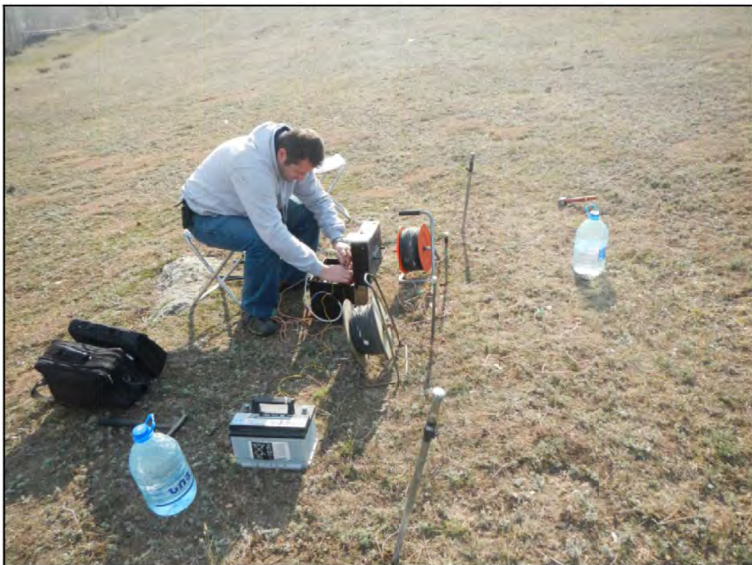
Figure 2.8: CYCLE-VPS digital electrical sounding station, field measurements
