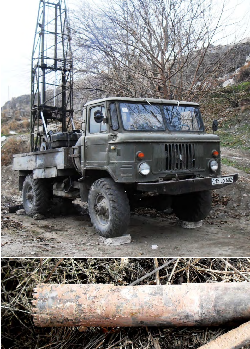
Figure 3.2.2: УТБ-50 drilling rig and the core bit 151 mm in diameter attached to the drilling rod
