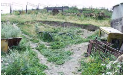
Sub scarp; 1.5m height, in the upper part of the displaced mass
