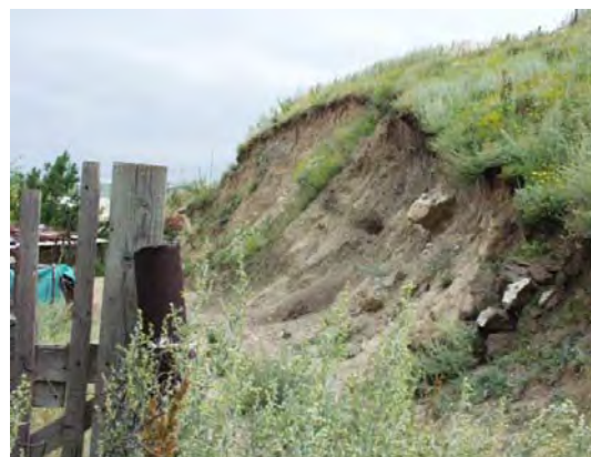
Sub scarp; 1.5m height, in the upper part of the displaced mass
