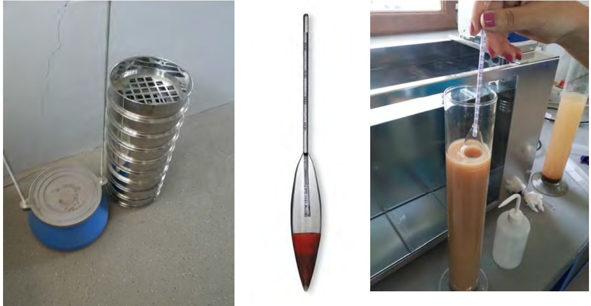
Fig.3.3.4. ASTM Sieves and ASTM 152-H-type Hydrometer
