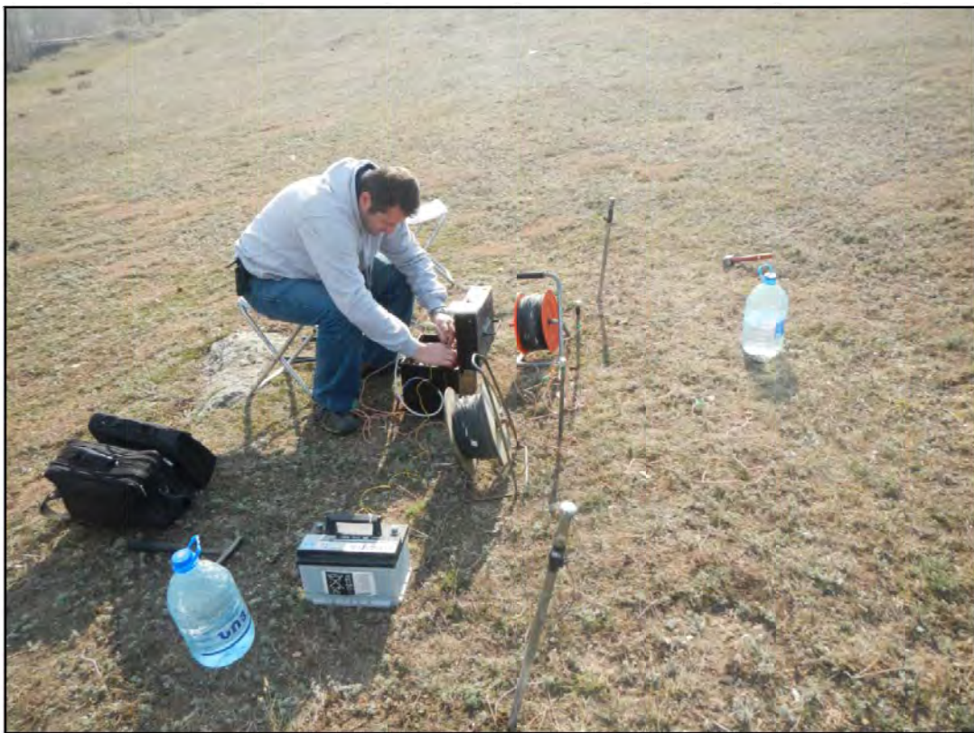
Figure 2.8: CYCLE-VPS digital electrical sounding station, field measurements
