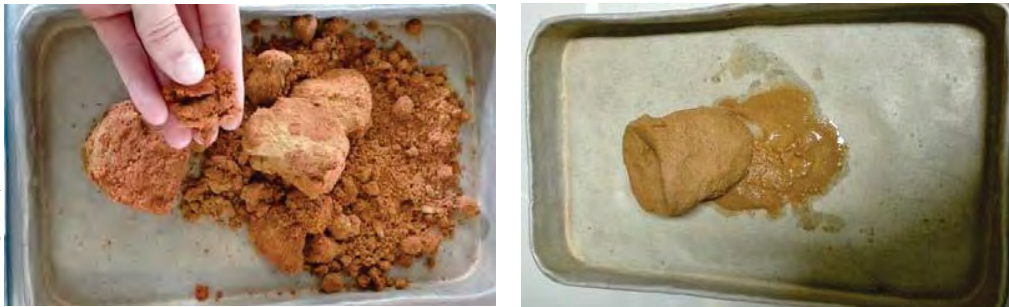
Figure 8 and 9 – Preparation of samples for triaxial tests.
