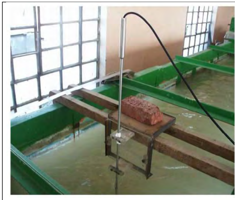
Figure 3-3.5 Flow velocity measuring equipment (micro current meter)
