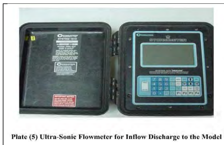
Figure 3-3.3 Inflow measuring equipment (ultrasonic flow meter)
