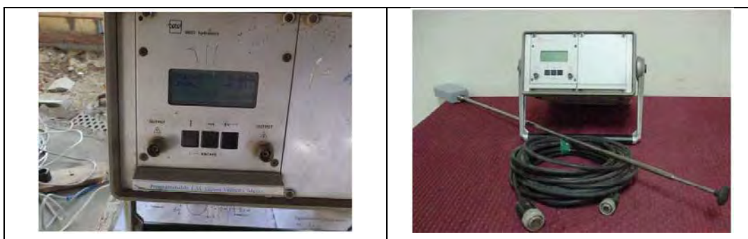
Figure 3-2.5 Flow velocity measuring equipment (micro current meter)
