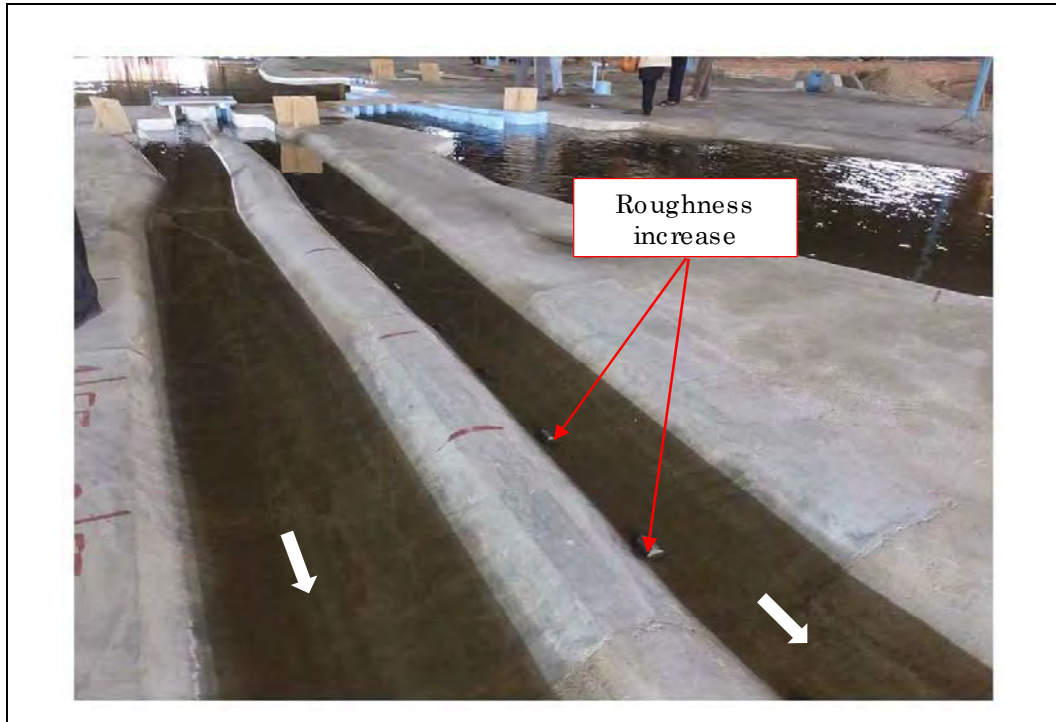
Figure 3-2.15 Increasing roughness on the downstream side of existing regulators (laving blocks)
