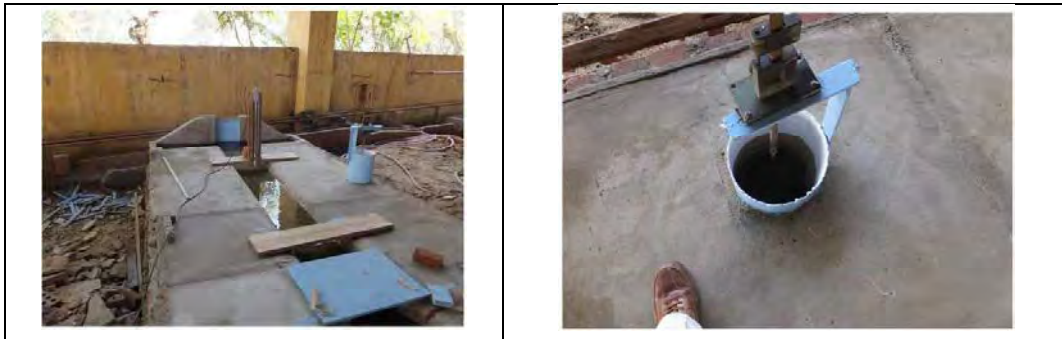
Figure 3-2.4 Water level measuring device (point gauge)
