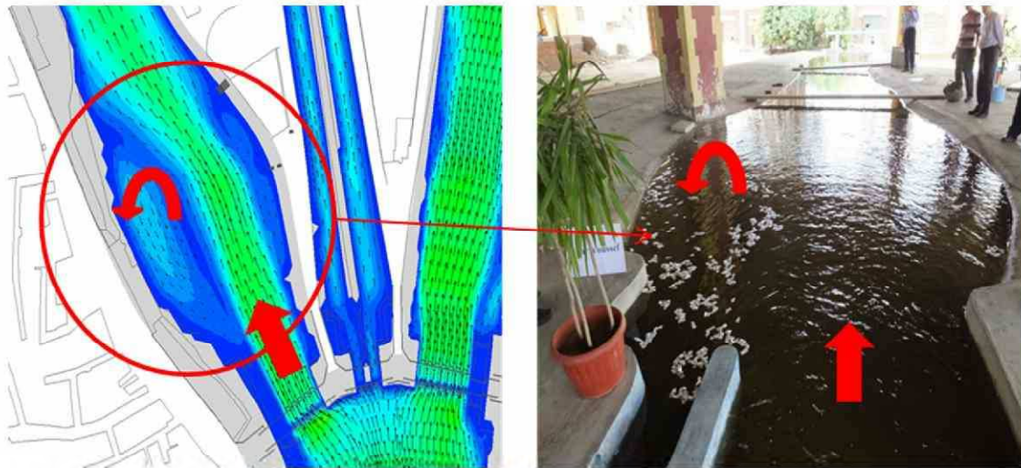
Figure 2-2.13 Comparison between the result of MMA and physical hydraulic model test (Bahr Yusef canal)
