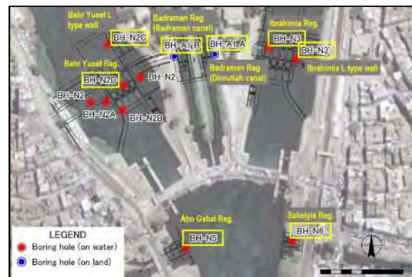
Figure12-1.3 Locations of borehole for design
