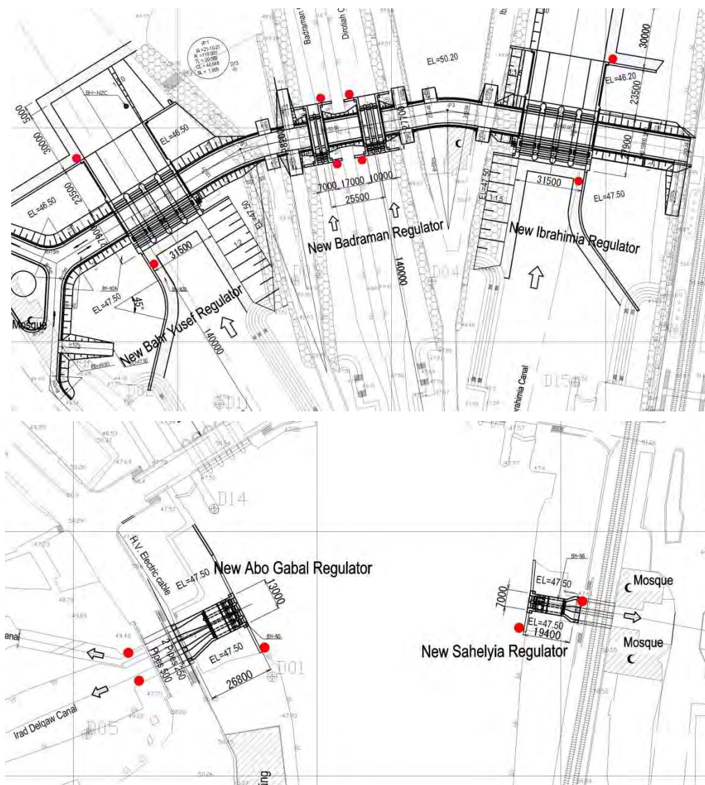
Figure17-1.1 Location of water gauges
