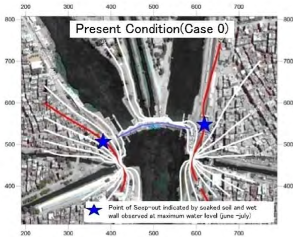
Estimated Water Head (ELm) ( at present condition, after construction of D/S140m & 150m Plan)
