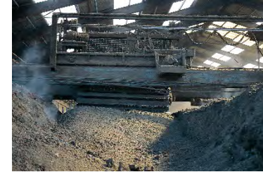
Cutback operations of the raw material by scoop type agitation equipment (24 hours)
