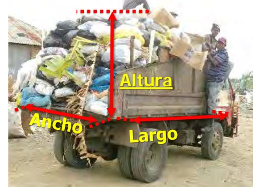
$$\text{Volume(M}^3\text{)} = \text{Ancho(m)} \times \text{Largo(m)} \times \text{Alto(m)}$$
