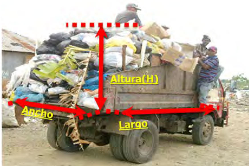
Figure 10 Analytical method for determining the measures of the equipment
