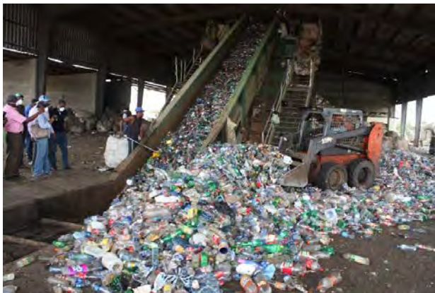
Intermediate treatment plant (compaction) of PET bottles in the Dump
