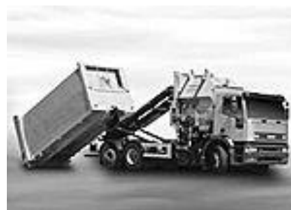
Photo 4 Solid waste loading system (2)
