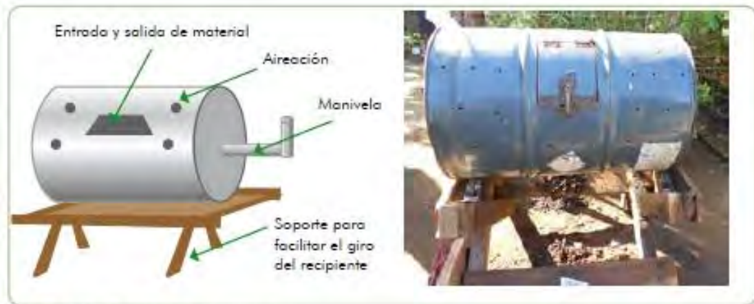
Figure 26 Closed composter for domestic technique.
