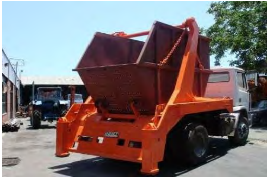
Special Dump Truck (Transfer station)
