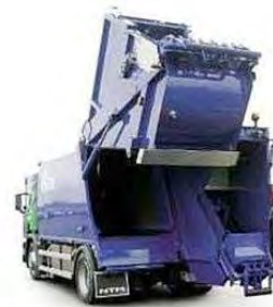
Photo 3 Solid waste loading system (1)
