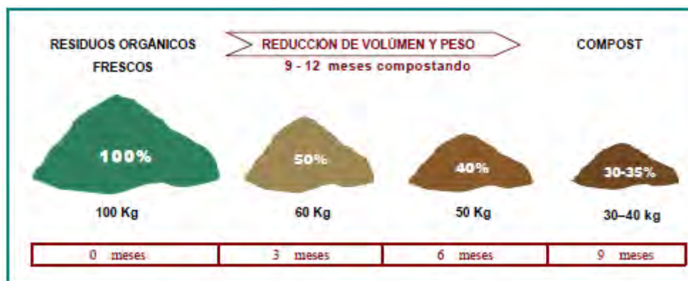
Figure 20 Decrease in weight and volume of organic waste during composting
