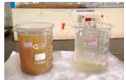
Wastewater at Nagasandra Sewerage Treatment Plant (Left: Before treatment, Right: After treatment)
