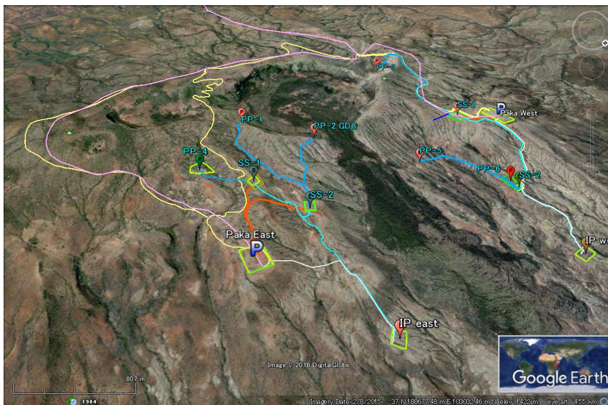
Fig. III-6.2 Possible layout of field development for Paka (View from the northeast)
