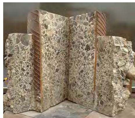
Steel pipe with outer ribs
