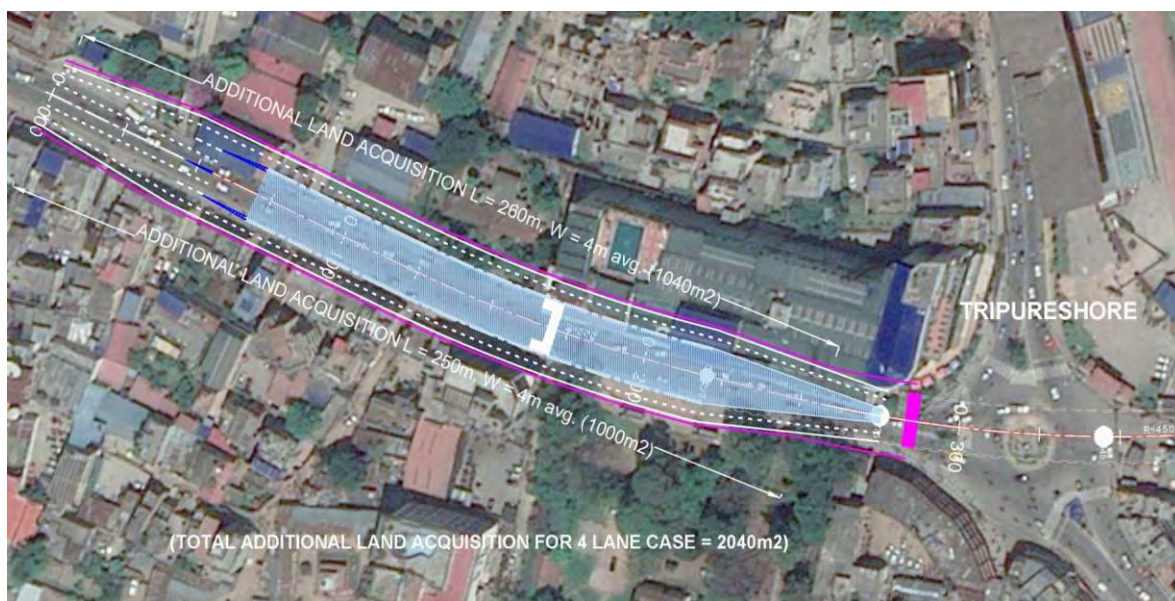
Figure 13.5.8 Additional Land Acquisition Area of 4-Lane Plan
