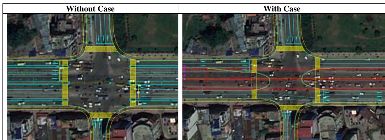
Figure 13.7.9 Lane Arrangement at New Baneshwor Intersection of Without Case and With Case
