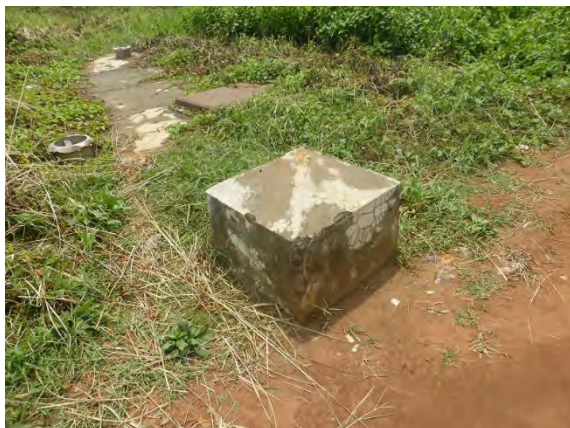
Control Point administrated by SOB Source: JICA Study Team
