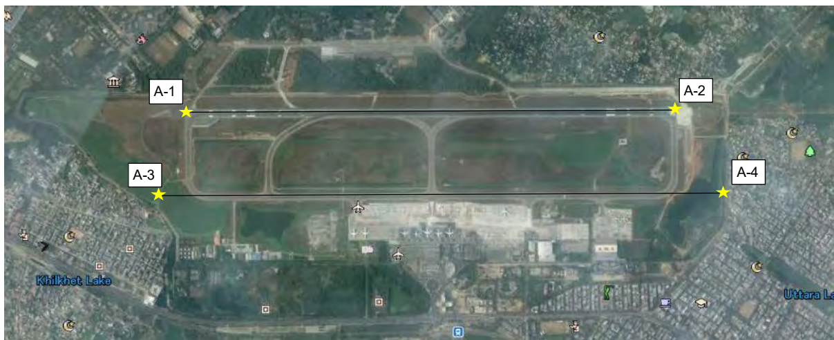
Figure 4-4 Location of Four Points for Control Survey
