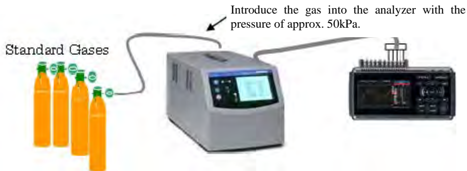
Figure 10-1 Introduce the gas into the analyzer with the pressure of approx. 50kPa.
