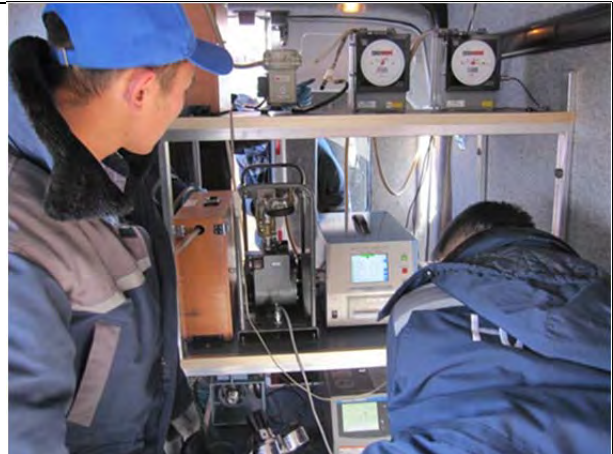
Flue gas Measurement on Measurement Vehicle
