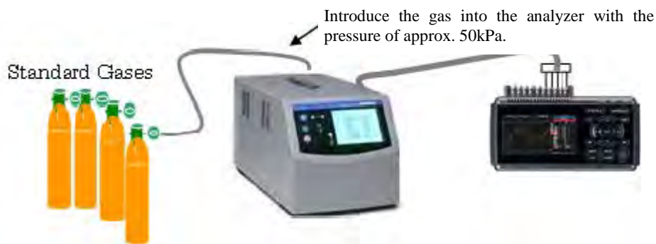
Figure 6-1 Introduce the gas into the analyzer with the pressure of approx. 50kPa.
