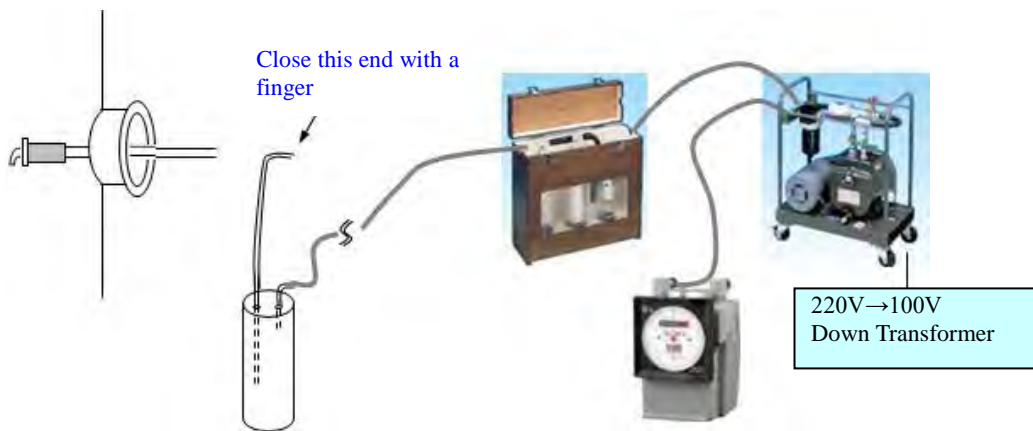
Figure 8-11 Leak Check on Sampling Tube
