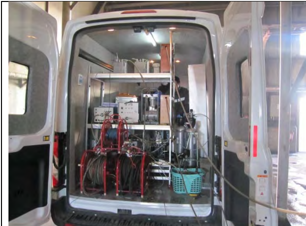
Flue Gas Measurement Vehicle
