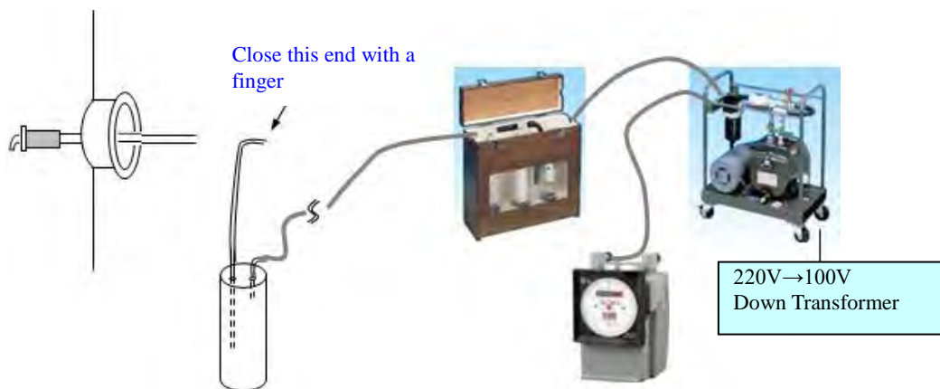
Figure 8-17 Leak Check on Sampling Tube
