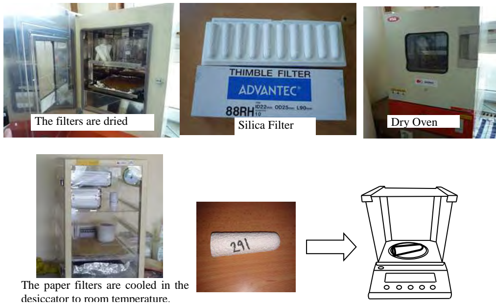
Figure 4-1 Preparation of the Dust Sampling Filter
