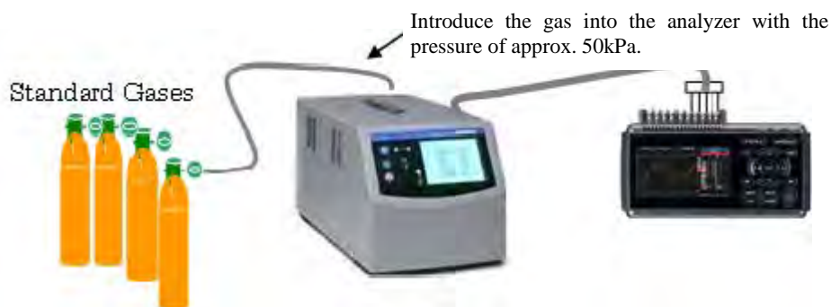
Figure 9-8 Introduce the gas into the analyzer with the pressure of approx. 50kPa.
