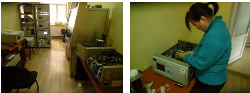
Figure 2.2-6 Images of O 3 Analyzer Periodic Maintenance at CLEM Reference Laboratory
