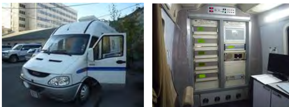
Figure 2.2-2 Image of APRD Mobile Air Monitoring Station and View Inside
