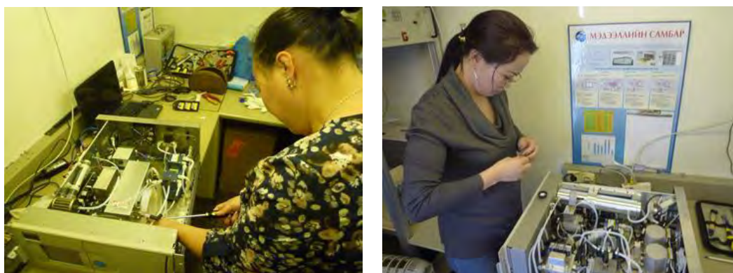
Figure 2.2-4 Images of Analyzer Major Part Replacement (Periodic Maintenance)
