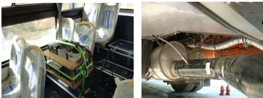
Figure 2.4-1 Measurement Using On-board Emission Measurement System
